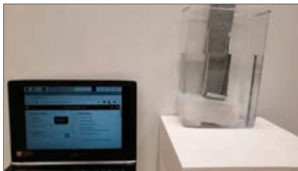
Figure 9. Raspberry Pi unit encased in Ecoflex (Figure 3) and submerged in water, communicating to and controllable from a PC via VNC over WiFi
