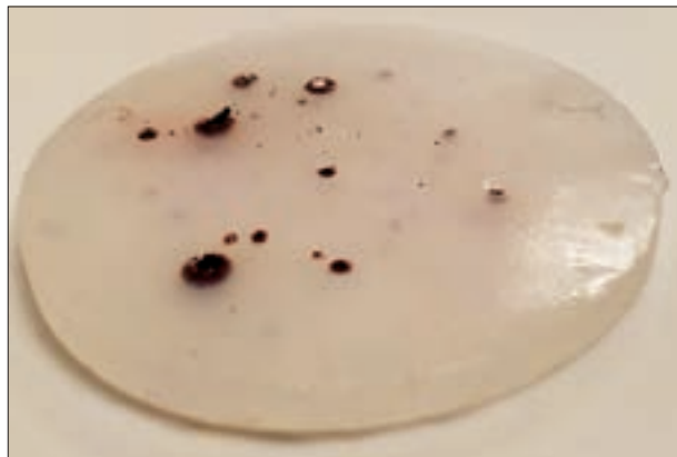
Figure 8. A small sample of Ecoflex with drops of red food dye, whose primary ingredients are water and propylene glycol, i.e., both polar molecules
