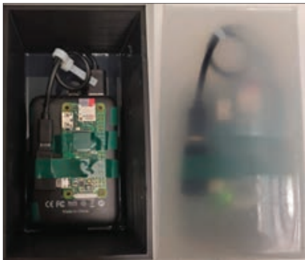
Figure 3. Before and after encapsulation of communication beacon electronics in Ecoflex
