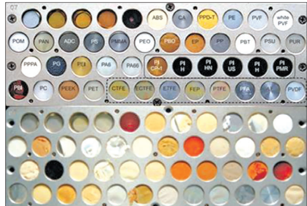
Figure 9. Pre-flight and post-flight photograph of the MISSE 2 PEACE polymers experiment tray
