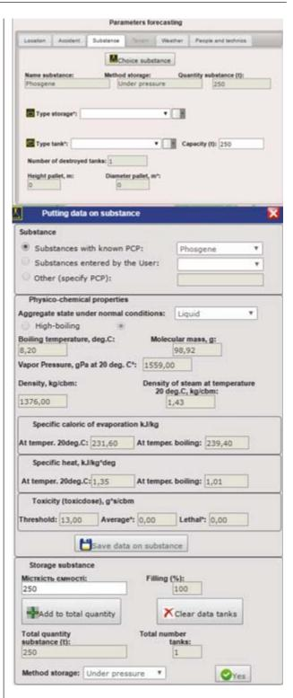
Fig. 2. Input windows of the Povitrya system for setting release scenario for screening models
