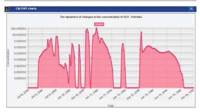
Fig. 8. Time series of calculated concentrations of SO<sub>2</sub> in air (ug/m<sup>3</sup>) visualized by Povitrya system
