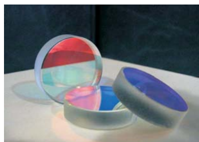
Fig. 2. Experimental specimens of the optical elements for the IR spectrum divisor with the multilayered coatings on the base of \text{MgF}_2\text{-LuF}_3 and \text{ZnS-GdS} composites (CDO "Arsenal")
