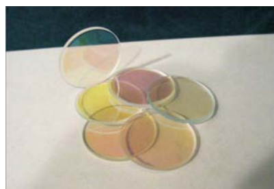
Fig. 3. Experimental specimens of the optical elements for the IR narrow-band filter with the multilayered coatings on the base of \text{MgF}_2\text{-LuF}_3 and \text{ZnS-GdS} composites (CDO "Arsenal")
