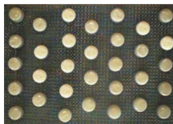
Fig. 1. Experimental samples of film forming material on the base of \text{MgF}_2\text{-LuF}_3 composite
