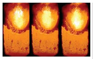
*Fig. 4.* Photos of gas bubbles generation and floating (arrows indicate the bubbles)
