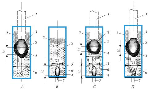
*Fig. 3.* The scheme of formation of the reaction zones at top (*A*), bottom (*B*), combined (*C*) and (*D*) oxygen blowing, 1 -lance; 2 -quartz plate; 3 -primary reaction zone; 4 -zone of reaction products; 5 -slag-metal phase; 6 -metal melt; 7 -bottom tuyere. h1, h2 - the depth of the primary reaction zone in upper and bottom parts of the model, respectively, D1 and D2 - the diameters of the primary reaction zones in upper and bottom parts of the model, respectively
