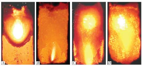
*Fig. 2.* Photo of reaction zones at top (*A*), bottom (*B*), combined (*C*) and (*D*) oxygen blowing with low voltage application of negative polarity
