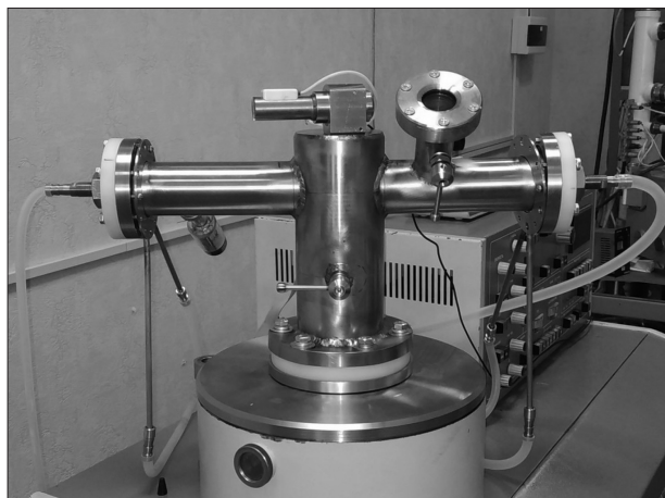
Fig. 4. Vacuum chamber with magnetron sputtering system
