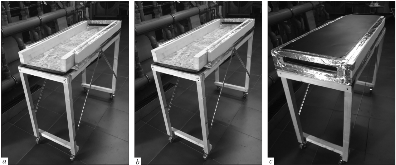
Fig. 2. Stages of manufacture of thermoactive roof panel: a – formation of timber framework; b – encased PCM; c – ready sample
