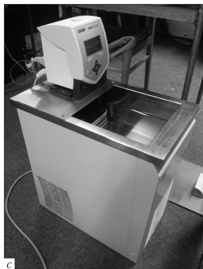
Fig. 5. Equipment used in the study: a – thermocouples; b – secondary metering device; c – calibration tank LAUDA ECO Silver
