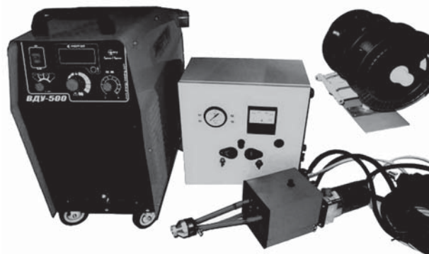
Fig. 2. Stationary arc spray gun kit for application of coatings
