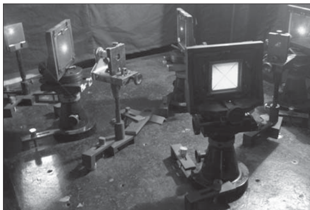
Fig. 2. Optical scheme of recording interference pattern on chips for SPR refractometer
