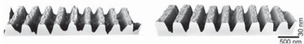
Fig. 5. AFM images of Au-chips with a period of 296.6 \pm 0.5 nm and an average relief depth of 13.5 \pm 2 nm (a) and 21.0 \pm 2 nm (b)
