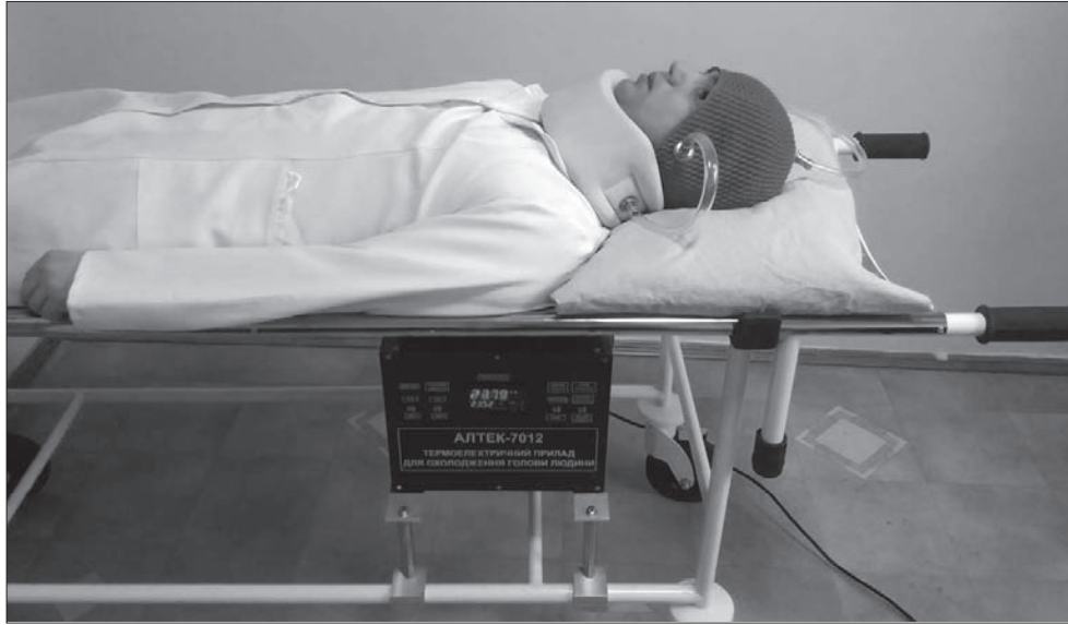
Fig. 7. Thermoelectric device for cooling of human head ALTEK 7012
