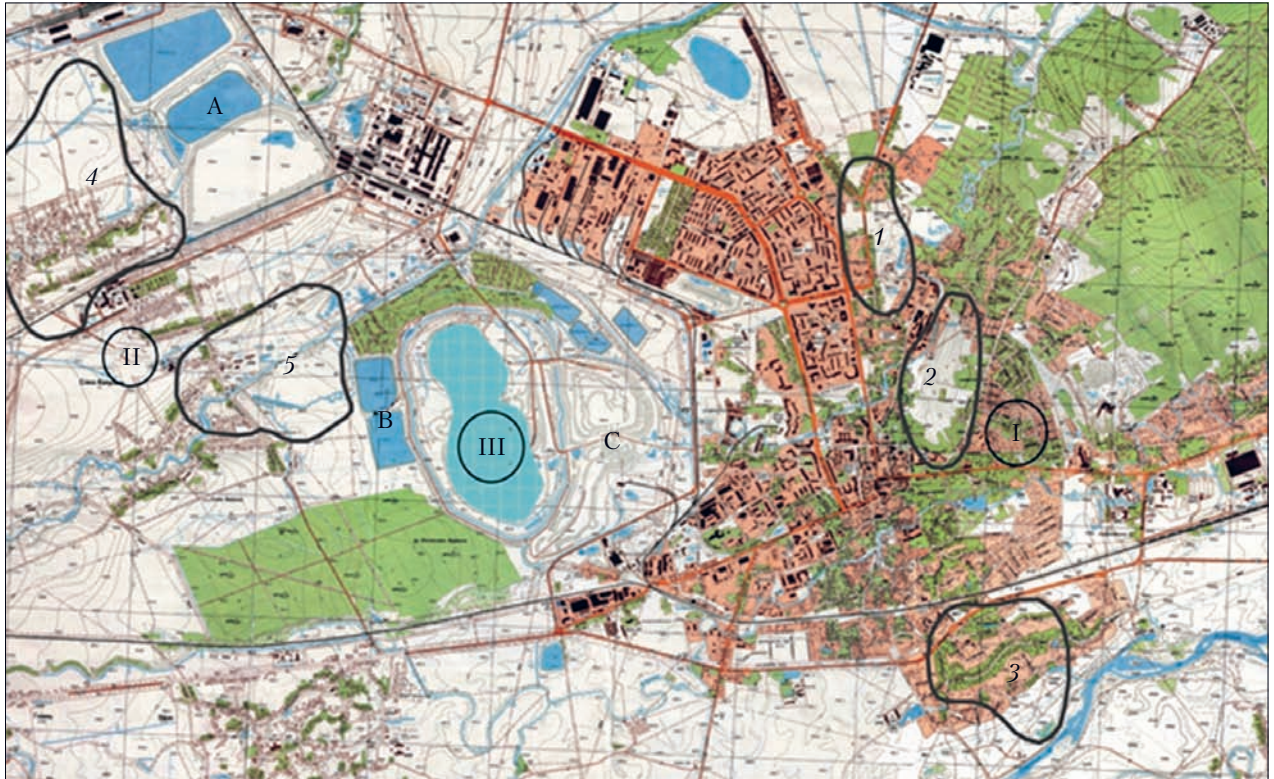
Fig. 3. The Kalush-Holyn deposit. Mines: I – Kalush, II – Nova Holyn, III – Dombrovsky quarry; mine fields: 1 – Northern kainite field, 2 – Central kainite field, 3 – Khotin sylvinite field, 4 – eastern Holyn field, 5 – Sivka-Kalush: A – tailings, B – accumulating basins, C – quarry dumps [24]
