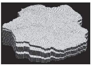
Geometry of water saturated layers of Chernihiv region with branched network of surface stream flows (the model covered area is 184 × 222 km)
