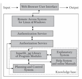
Fig. 4. Client-server architecture of Inpartool\_pg
