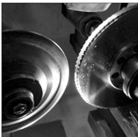
Fig. 4. Finishing of the roller on the opto-grinding machine
