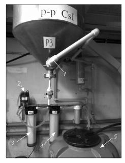
**Fig. 2.** The view of the experimental-industrial node of CsI purification by filtration through cartridge filters filled with magnesium and carbon: 1 - heat-exchange apparatus (ti-tanium); 2 - metering pump; 3 - Mg-filled cartridge filter; 4 - activated carbon-filled cartridge filter; 5 - capacity for the filtered solution
