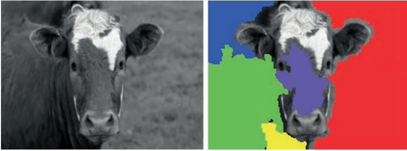
Fig. 3. Results of texture segmentation of a grayscale image (left part of the figure). The right part of the figure shows the 5 largest texture segments extracted by the model (in different colors)
